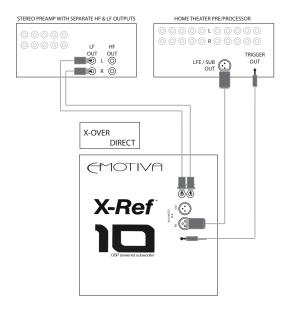
A typical installation, with a single X-Ref 10 DSP Powered Subwoofer providing bass enhancement for both a stereo system and a hometheater pre/processor
